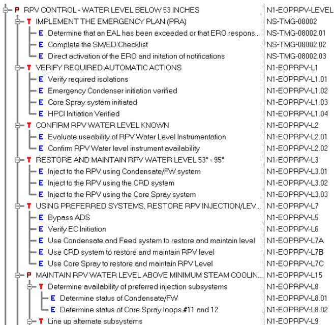
In this model the "Phase" organizer represents the beginning point for the RPV LEVEL portion of the EOP (in reality, all legs of an EOP are entered concurrently) while the tasks represent discrete operating results or potential major nodes (resulting in branching to another procedure) and the elements the actions that must be completed or evaluated before progressing to the next major transition point.
